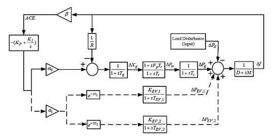
Figure 2. Dynamic model of single-area LFC system with EVs and communication delays.
