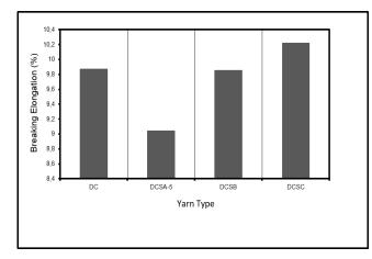
Figure 12. The average breaking elongation results of Group-II yarns.
