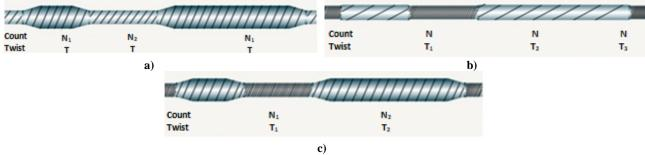
Figure 2. Basic slub (a), Multi-twist slub (b), Multi-count slub (c).
