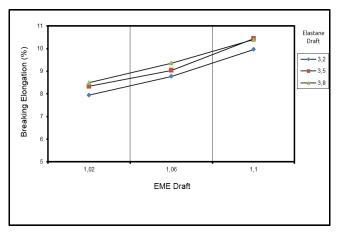
Figure 11. The average breaking elongation results of Group-I yarns.
