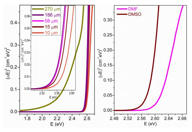
Fig. 5.  $(\alpha E)^2$  curves vs. photon energy (E) of BHYC for different molarities (a) and solvents (b)
