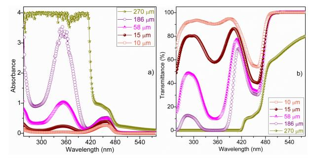
Fig. 3. a) Absorbance and b) transmittance spectra of BHYC solutions for 10, 15, 58, 186 and 270 µM molarities
