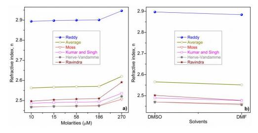
Fig. 6. Refractive index (n) curves of BHYC for different molarities (a) and solvents (b)
