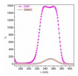
Fig. 7. Electrical susceptibility ( $\chi_c$ ) curves vs.  $\lambda$  of BHYC for DMF and DMSO solvents
